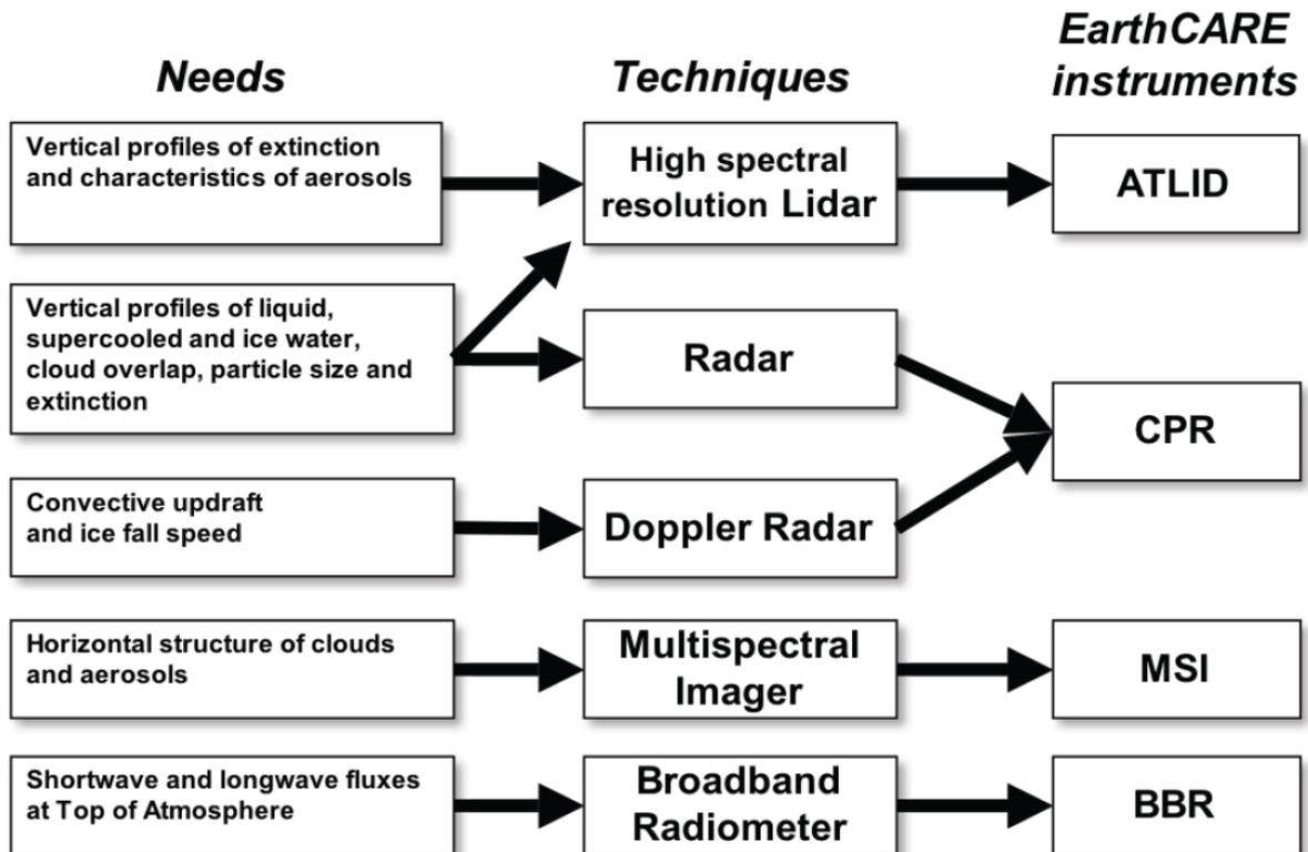
Figure 1 Relationship between target geophysical parameters and instruments
