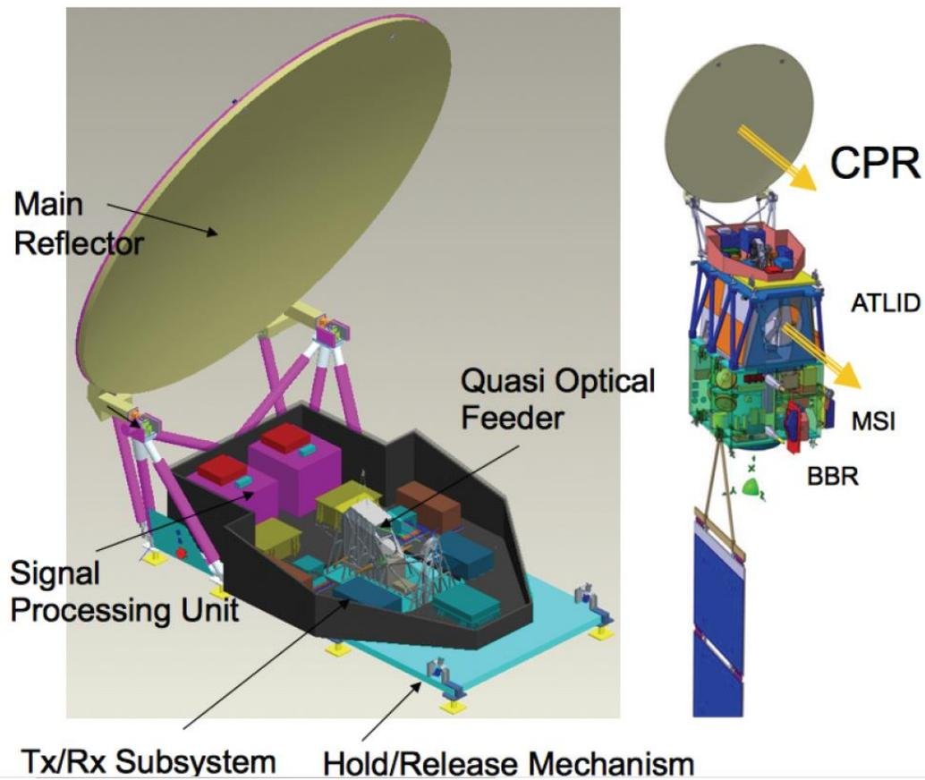
Figure 2. Outlook of CPR and EarthCARE satellite
