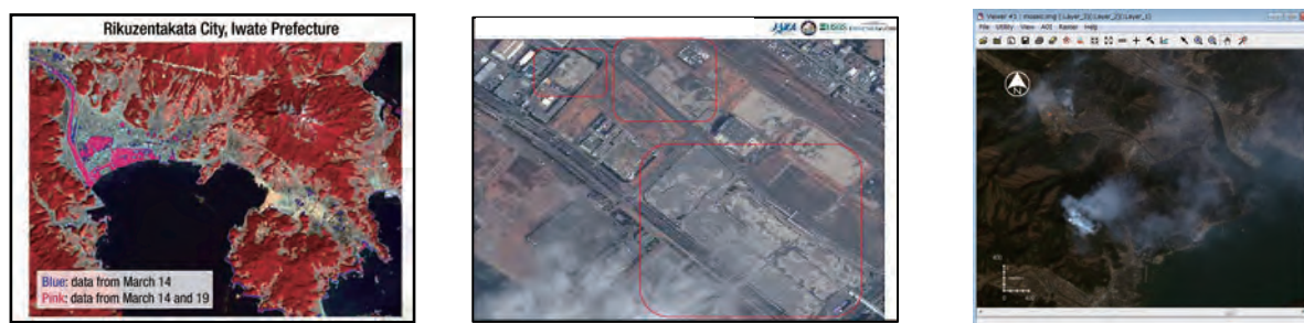
Figure 2.1-53 Image of flooded areas extracted from AVNIR-2 data (left), identification of liquefaction areas (middle) and identification of a wildfire (Otsuchi Town, Iwate) (right)
