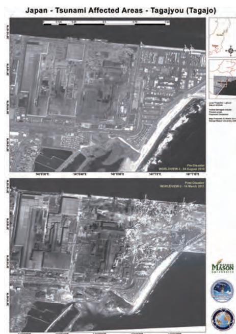
Figure 2.1-36 Example of image analysis products produced by overseas institutions (George Mason University.) Pre- and post-disaster images of tsunami-affected areas in Tagajo City, Miyagi, taken using a high-resolution optical sensor Images used: Worldview-2 (top: observation before disaster on August 4, 2010; below: observation after disaster on March 14, 2011)
