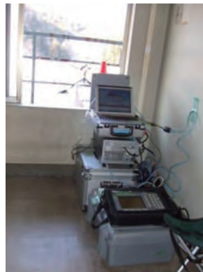
Figure 2.2-18 Communication equipment installed (left: 90 cm \phi portable antenna; center: portable communication terminal equipment; right: portable generators)
