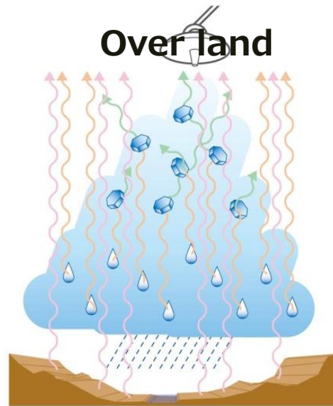
Passive microwave sensor 19GHz (Low-frequency channel)
