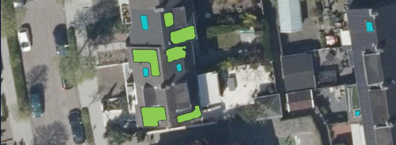
Roof windows and solar panels
