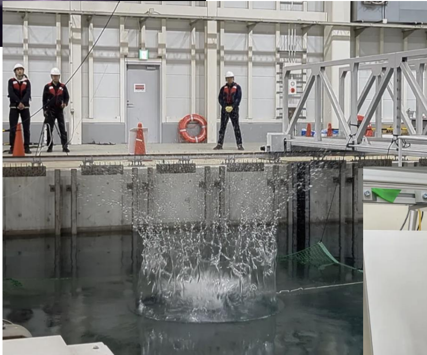
Reentry capsule splash down test
